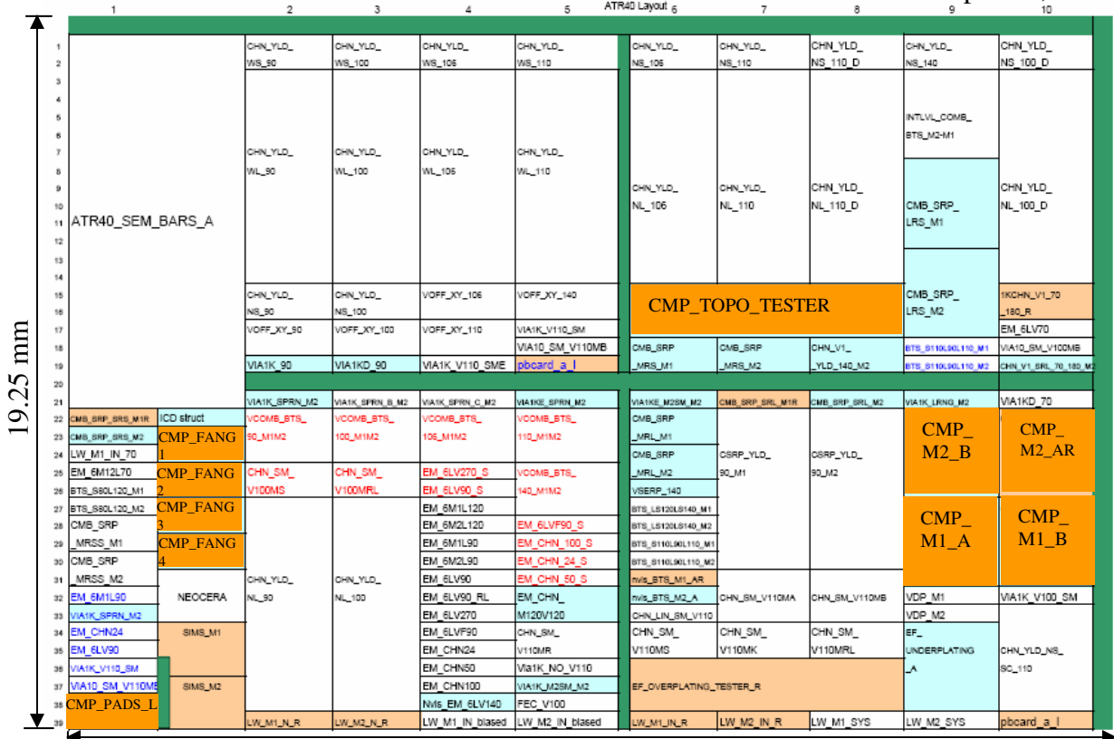
ATR-40 Cu/CORAL Mask Floor Plan (CMP test structures highlighted in orange)
